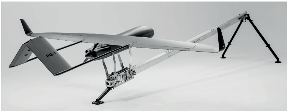
Figure 3. Fixed-wing drone on the launcher Source: (UST, 2018)
